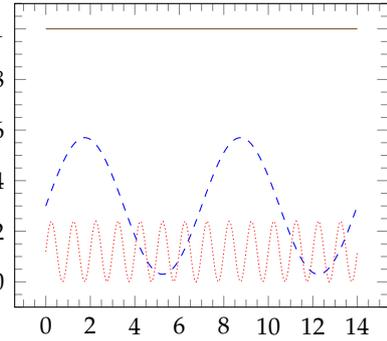
Figure 1: Diurnal and synoptic variations of wind and solar power generation  $G_{N,w}(t)$  --- and  $G_{S,s}(t)$  ·····, and a constant load (all in per-unit)  $L(t)$  —.
